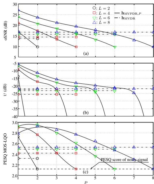
**Fig. 1.** Performance of  $\mathbf{h}_{\text{MVPDR},P}$ , as a function of  $P$ , and the single-channel MVDR filter in a car noise environment with different filter lengths: (a) oSNR, (b) speech distortion, and (c) PESQ score. The input SNR is 10 dB.
