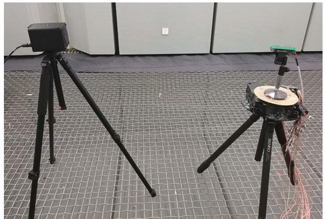
FIG. 10. (Color online) The experimental setup for measuring the real beam patterns.
